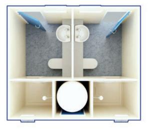
A truly high quality unisex changing facility. As with all of our units, the internal specification makes it equally suitable in the event, leisure or construction industries. The unit is divided into two equal cubicles. Each houses a powerful shower, water flushing toilet and a wash hand basin. These electric showers avoid the inherent dangers of gas.
