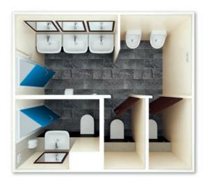
Our Toilet Block with its LED lighting offers a bright and inviting space. Its 2-plus-1 layout has two toilets, two urinals and three wash hand basins on one side and a separate partitioned toilet with wash hand basin on the other. A thermostatically controlled, low energy tubular heater ensures the environment stays warm and efficient extractor fans help each area remain fresh.
